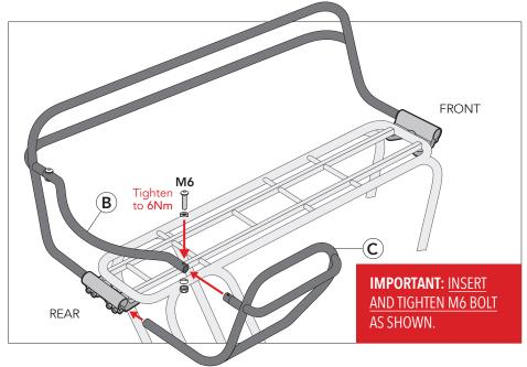
2. Insert lower end of three quarter rail (C) from the right side into the rear clamp until it comes to a stop while connecting the upper end to the rear rail (B) as shown. Insert and tighten M6 bolt, spacers and nut as shown to ensure secure connection between rail (B) and three quarter rail (C).
