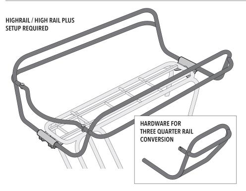
**IMPORTANT:** *Notes to mechanic:* See Instructions. Install Benno three quarter rail conversion kit only on compatible Benno high rails or high rail plus and use only pre-drilled holes and fittings. Do not mount to damaged clamps, racks or rails. Do not modify clamps, racks or rails, change position or drill new holes as this will void any warranties and/or claims for liability.
