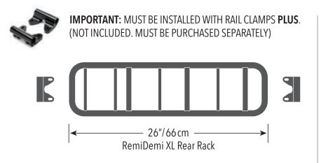
**IMPORTANT:** Notes to mechanic: See Instructions. Install Benno rail clamps and rails only on compatible Benno rear racks and use only pre-drilled holes and fittings. Do not mount clamps and rails to damaged racks. Use only original Benno rails with the Benno rail clamps. Do not modify clamps, racks or rails, change position or drill new holes as this will void any warranties and/or claims for liability.
