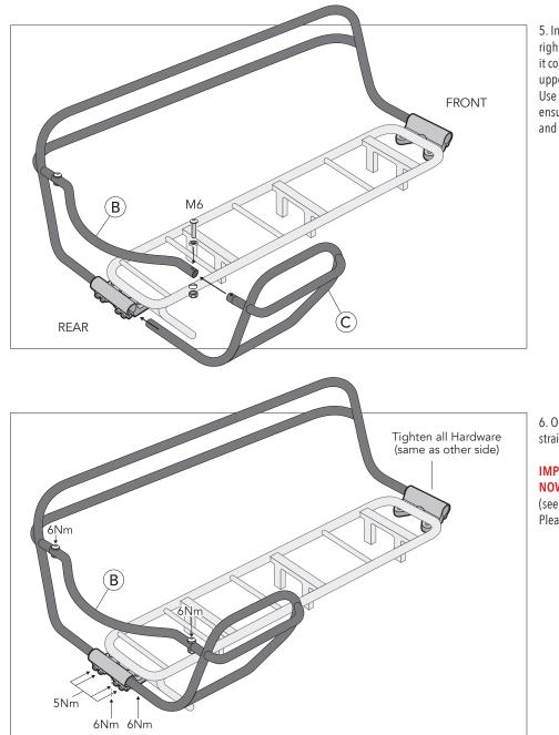
5. Insert lower end of right rail (C) from the right side into the center of the clamp until it comes to a stop while connecting the upper end to the rear rail (B) as shown. Use M6 bolt, spacers and nut as shown to ensure secure connection between rail (B) and rail (C).
