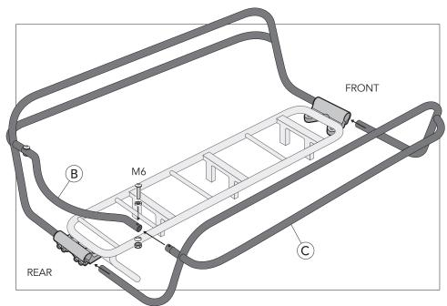
5. Insert both lower ends of right rail (C) from the right side into the center of the clamps until they come to a stop while connecting the upper end to the rear rail (B) as shown. Use M6 bolt, spacers and nut as shown to ensure secure connection between rail (B) and rail (C).
