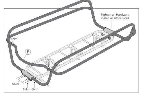
6. Once all pieces are installed, adjust and straighten rails and clamps as needed.
