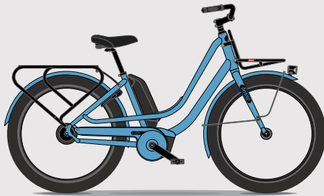
Sturdy rear rack with 85lbs/40kg max load capacity.
