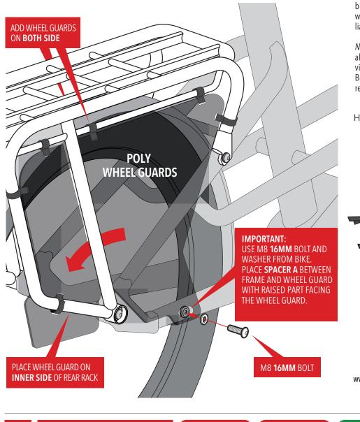
**IMPORTANT:** Notes to mechanic: See Instructions. Install Benno 46er Poly Wheel Guards only on compatible Benno 46er models. Use only original (included) hardware and pre-drilled holes and fittings. Do not mount 46er Poly Wheel Guards to damaged bikes or racks. Do not modify wheel guards, racks or bikes, change position or drill new holes as this will void any warranties and/or claims for liability.
