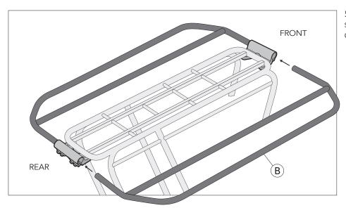
5. Insert both ends of rail (B) from the right side all the way into the center of the clamps until they come to a stop.
