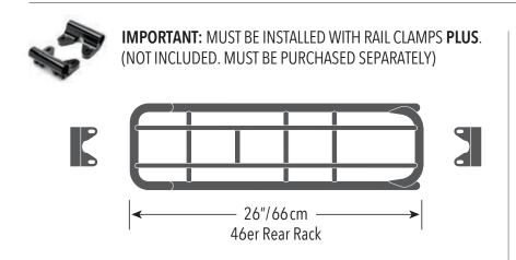
**IMPORTANT:** Notes to mechanic: See diagram. Install Benno rail clamps and rails only on compatible Benno rear racks and use only pre-drilled holes and fittings. Do not mount clamps and rails to damaged racks. Use only original Benno rails with the Benno rail clamps. Do not modify clamps, racks or rails, change position or drill new holes as this will void any warranties and/or claims for liability.
