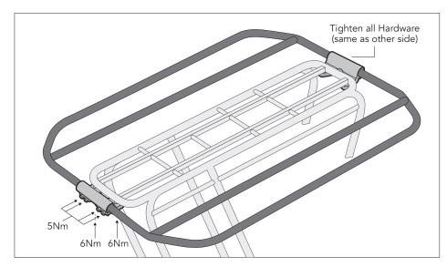
6. Once all pieces are installed, adjust and straighten rails and clamps as needed.
