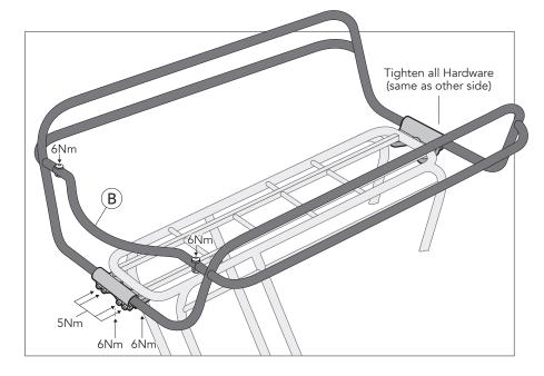
6. Once all pieces are installed, adjust and straighten rails and clamps as needed.
