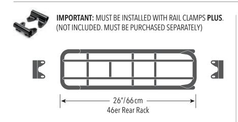
**IMPORTANT:** Notes to mechanic: See diagram. Install Benno rail clamps and rails only on compatible Benno rear racks and use only pre-drilled holes and fittings. Do not mount clamps and rails to damaged racks. Use only original Benno rails with the Benno rail clamps. Do not modify clamps, racks or rails, change position or drill new holes as this will void any warranties and/or claims for liability.
