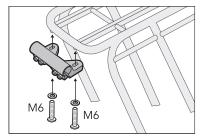
3. Insert the two M6 bolts through the slotted holes of the clamp and screw into the fittings on the underside of the rack. HAND-TIGHTEN BOLTS SLIGHTLY – CLAMPS STILL NEED TO BE ABLE TO MOVE.
