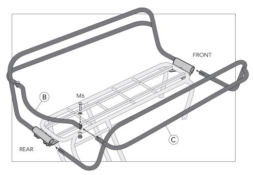
5. Insert both lower ends of right rail (C) from the right side into the center of the clamps until they come to a stop while connecting the upper end to the rear rail (B) as shown. Use M6 bolt, spacers and nut as shown to ensure secure connection between rail (B) and rail (C).
