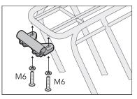
3. Insert the two M6 bolts through the slotted holes of the clamp and screw into the fittings on the underside of the rack. HAND-TIGHTEN BOLTS SLIGHTLY – CLAMPS STILL NEED TO BE ABLE TO MOVE.
