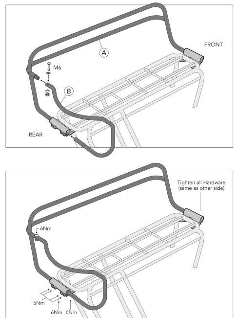
5. Insert the lower end of the rear rail (B) from the right side into the center of the rear clamp until it comes to a stop while connecting the upper end to the left rail (A) as shown. Use M6 bolt, spacers and nut as shown to ensure secure connection between rail (A) and rail (B).
