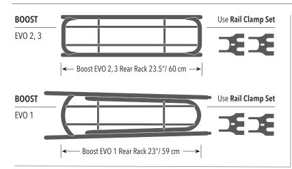
**IMPORTANT:** *Notes to mechanic:* See diagram. Install Benno Rail Clamps and Rails only on compatible Benno Boost Rear Racks and use only pre-drilled holes and fittings. M5 bolts are to be tightened to 5Nm and M6 bolts to 6Nm. Do not mount clamps and rails to damaged racks. Use only original Benno Rails with Benno Rail Clamps. Do not modify clamps, racks or rails, change position or drill new holes as this will void any warranties and/or claims for liability.
