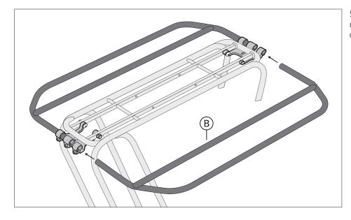
5. Insert both ends of rail (B) from the right side all the way into the center of the clamps until they come to a stop.
