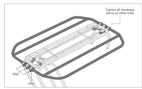
6. Once all pieces are installed, adjust and straighten rails and clamps as needed.
