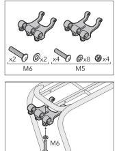
1. Ensure correct hardware count before installation. Separate the 2 larger M6 bolts and washers from the 4 smaller M5 bolts, washers and self-locking nuts.
